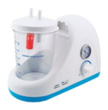
Main Technical Specifications Piston pump Suction pump Ultimate negative pressure ≥ 0.075MPa Regulating scope of negative 0.02MPa  $\sim$  ultimate pressure negative pressure value Air exhausting speed ≥18L/min Reservoir 1000ml, 1pc Power supply AC220V / 110V, 50Hz / 60Hz Input power 90VA Noise ≤65dB(A) Dimension 335mm×150mm ×240mm
